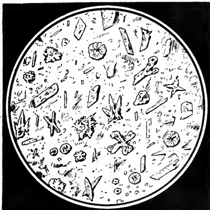
Fig. 2.—Magnified transparent layer of crystalline matters from dried films of pulp froth; the distension of which, in solution, enables the bubbles to form. Actual diameter of space about 1-24th of an inch.
